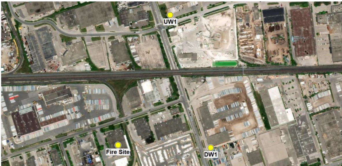
Figure 1. Mobile TAGA Monitoring sites. UW1, DW1 and Fire Site indicate the upwind monitoring location, the downwind monitoring location, and the location of the active fire.
